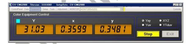
CV-CMG2000 can display the measured value on the interface like above.
